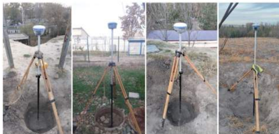
Fig. 2. Field measurement work at points of the Frame Network (FN).
