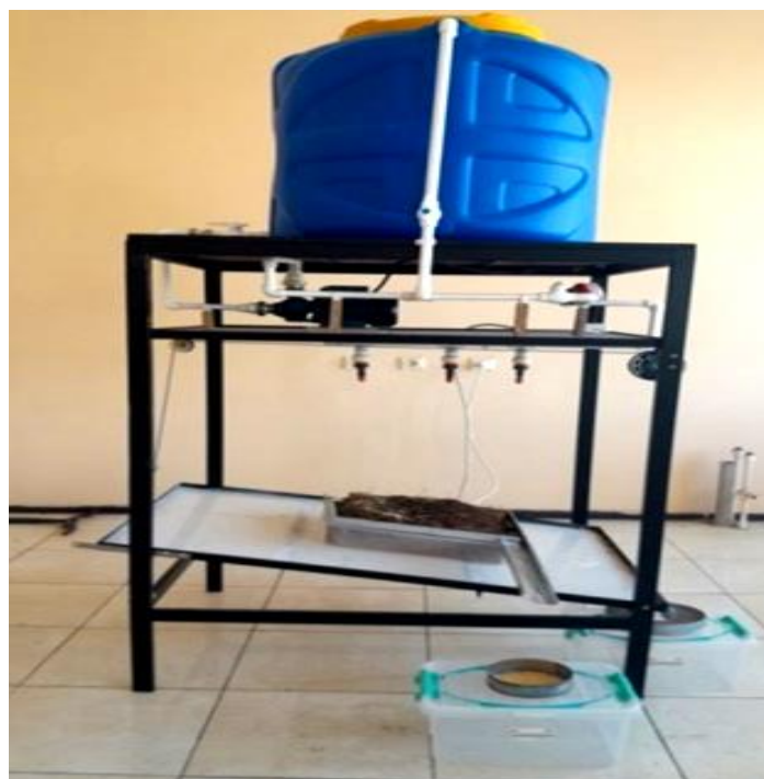
Figure 1: Laboratory device “Model of artificial sprinkling”
